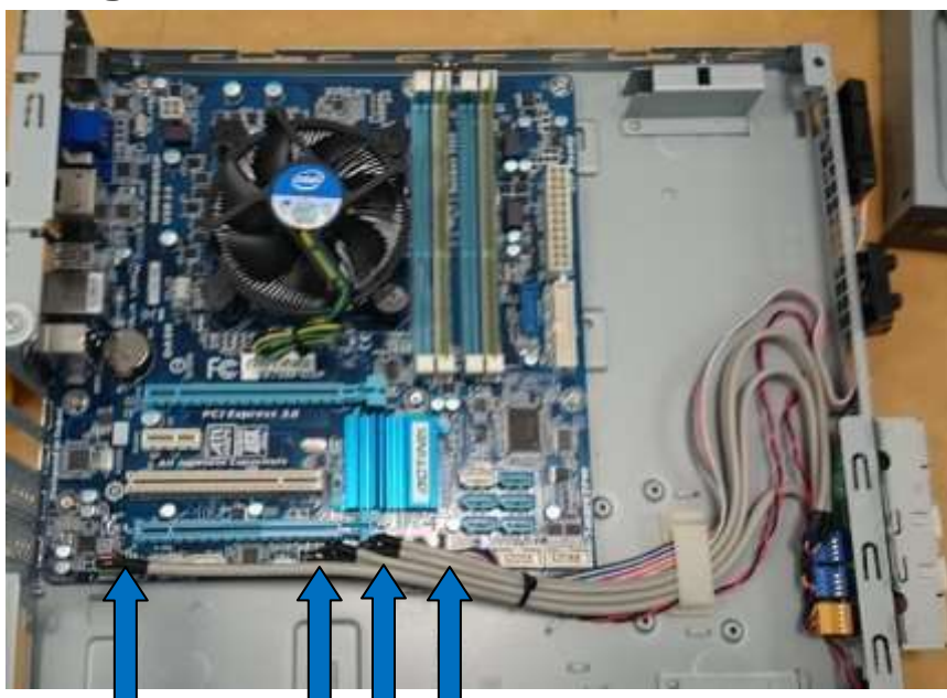
8.1 Disconnect the identified signal cables from the motherboard
